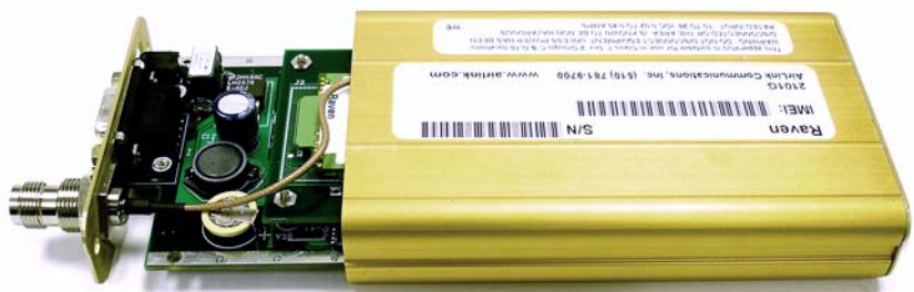
FIGURE B-2. Modem Partially Slid from Case
