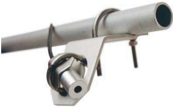
The SI-111 is mounted to a CM204 crossarm via the CM230; the CM230 allows the sensor to be pointed at the surface of interest.
